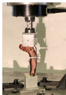
Figure 1. Set up of mandible with distractor in place during a compression test
